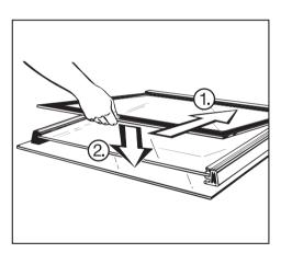
Insert the inner pane with the printed text facing downwards.
